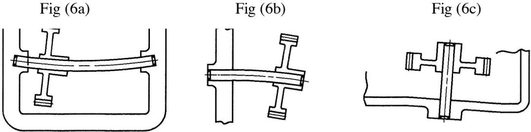
One type of gear assembly is particularly sensitive to misalignment due to deflections under load. The planet gear in planetary gear arrangements is often supported by a cantilevered shaft, which may be of limited diameter to reduce bearing friction losses. The web portion of the planet carrier, connecting the planet shafts, may be of reduced thickness to save space. The combined deflection of these features under load, pictured in figure (7) contributes to gear mesh misalignment.
