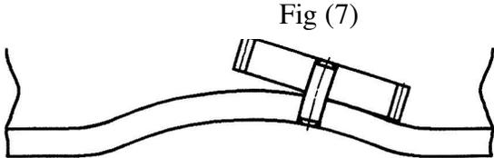
Then the gears themselves may have tapered faces, figure (8a), which will misalign and/or tapered bores which will allow movement under load. Distortion in the web creates wobble of the gear teeth to both sides of center, figure (8b).
