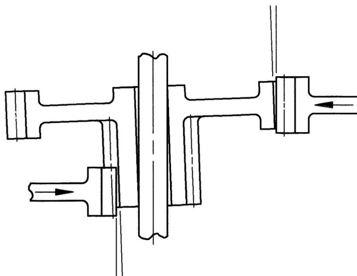
Offset Tooth Loading on Driving & Driven Gears
