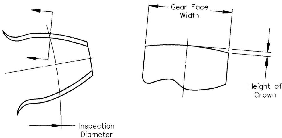
A simple equation may be used to determine the height of crown needed:
